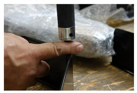
3. The bolt to attach should go in the second hole from the top of the round or square rod as shown below. Any higher or lower and you run the risk of having the deflector drag too much or not work properly.
