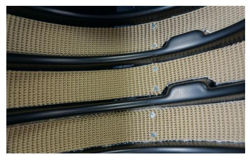
5. Finally, insert 2 more screws into the other side of the strip, in the same way as step 3, and cut any excess rubber that overlaps (Old holes may be used, if worn, route new ones)
