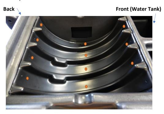
3. Insert rubber strips & use drill to secure each strip using 2 screws on one side (Old holes may be used, if worn, route new ones)
