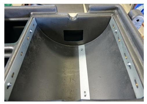
\*\*If replacing guide set on 50G Superwash, insert black rubber pad before starting Step 2\*\*
