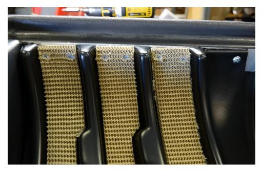
4. Next, insert 2 screws, using a drill, onto the bottom/center of the strip to secure it to the tank (Old holes may be used, if worn, route new ones)
